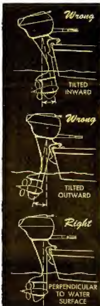
Note how wrong motor tilt affects the performance of boat. Motor in lower photo is tilted correctly
